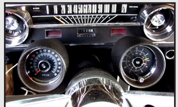
Figure 2: Rally Pac positioned and mounted
