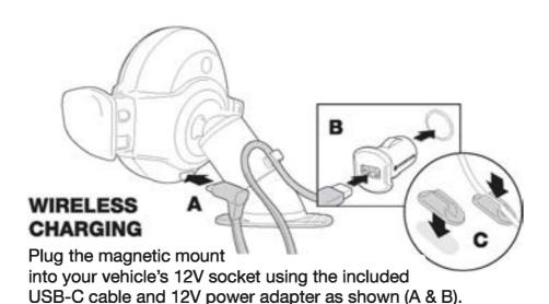
**Optional:** Attach the included adhesive clips (C) to the dash or console to secure the cable.
