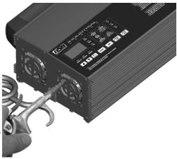
out quickly. If the fans fail, the charger may overheat and the thermal protection of the charger will shut it down.
