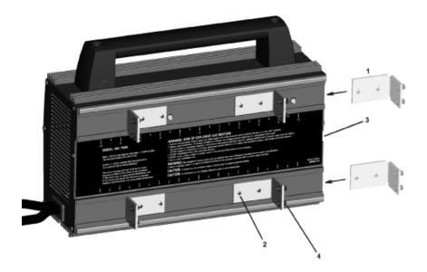
This charger can be operated on a stable surface either upright or lying down (brackets not installed). Rubber strips have been provided to help prevent scratching and denting of the channels. If you would like to permanently mount the charger, use the following instructions:
