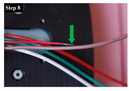
Note: The side marker light must be connected to the driving light signal of the tail light which is the brown wire. The following steps will instruct you to splice the red side marker wire to the brown driving light signal.
