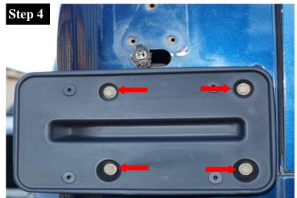
Please note that the OEM license plate mount has to be removed and lowered to install the Savvy Tail Lights. Savvy has made a license plate relocation bracket for purchase should you require it. The low profile of the Savvy Tail Light housing eliminates the license plate lighting. If a license plate lighting is required you may purchase our LED bolts or other options in the market.
