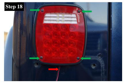
Install (4) #6 - 32 x 5/8" Pan Head Machine Screws (E) as shown in the green arrows. Start all 4 screws before tightening to snug. **Do not overtighten to avoid cracking the tail light lens.**
