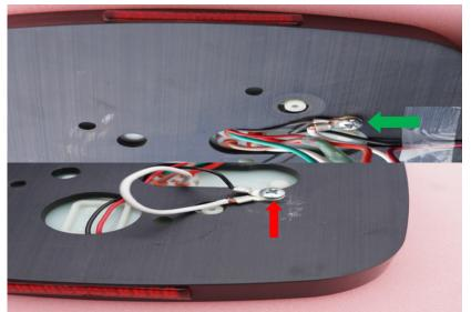
Crimp a #6 Ring Terminal to the white wire and install both the side marker, license plate lighting and tail light lens grounds to the housing using (1) 6 - 32 x 1/4" Pan Head Machine Screw (F) on the threaded hole closest to the side marker lens.
