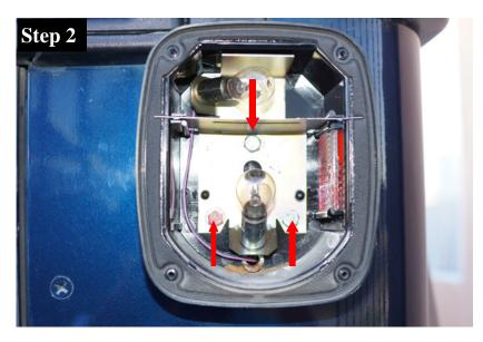
Next remove the three screws that retains the OEM tail light housing to the Jeep tub (red arrows).
