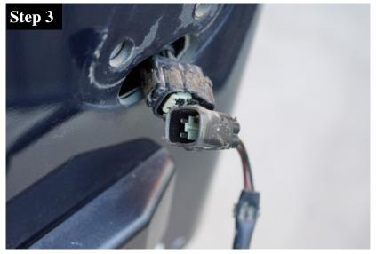
Carefully pull the tail light housing out and disconnect the housing plug. You may have to work the connector loose from the emission hardware behind the jeep tub.
