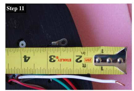
The white wire on the tail light lens must be grounded to the tail light housing. Measure and cut the white wire to 4 inches.
