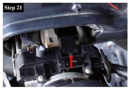
Grab the OEM flasher relay and pull in the direction as shown by the red arrow.
