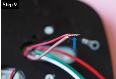
Strip about 5/16" off the insulation for both brown and red wires and twist together as shown in blue arrow.
