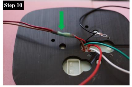
Using a 16-14 Ga Heat Shrink Crimp Solder Butt Connector (J), crimp the side marker power (red) wire to the brown tail light lens wire to one side of the butt connector and the 12in. 20 AWG Primary Red Wire (G) and remaining brown tail light lens wire to the other side of the butt connector (green arrow).
