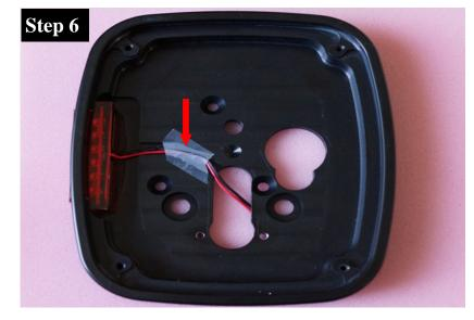
The Tail Light Housing includes a LED side marker light that must be tied into the housing ground plane and the running light power signal. These steps will be performed later on.
