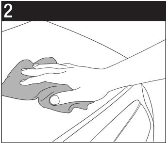
Step 2: Clean surface of vehicle which will be in contact with rack.
