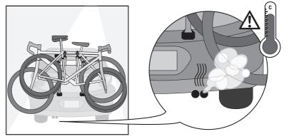
Install bike in rack cradles as shown. Lower anti-sway strap on arm should be positioned at the rear of the bike. Close straps and pull tight. Heaviest bikes should be installed closest to vehicle. Note: be aware of bicycle tire position in relation to vehicle exhaust. Be sure bike tires are at least 12" from ground. Do not open trunk or hatch with rack and/or bikes installed.
