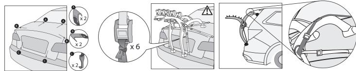
Install rack hooks in locations as shown. Hooks are labeled upper, side and lower. Upper hook straps can route through channels in upper legs. Reference fit guide on website for recommended upper leg strap position. Tie off all straps as shown once thoroughly tightened.
