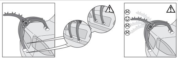
Place lower rack feet on bumper. Some vehicles require the feet to be on the trunk lid, refer to website fit guide for proper feet placement on your vehicle. Place upper feet in center of trunk lid or center of rear window. Raise rack arms as shown. Note: bike cradles furthest from vehicle should be highest from the ground.
