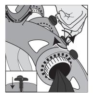
Turn knob on rack arm counterclockwise to loosen rack arm. Slide arm to center of aluminum tube and open arms as shown, slide arm back over aluminum tube spline. Tighten knob by turning clockwise.
