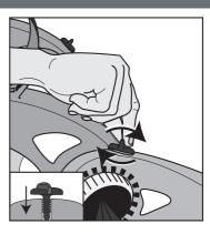
Turn knob counterclockwise on outer leg knob to loosen leg as shown. Remove leg from spline and reinstall on spline at desired position. Refer to page 6 to determine optimal rack orientation. Tighten knob.
