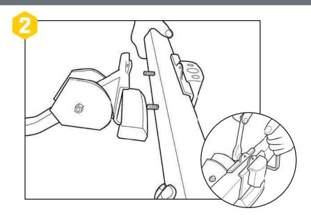
EN Lay horizontal bar on to receiver plate, lining up front plate with bar and receiver. Secure with bolts & nuts, using 17mm (9/16") wrench and 8mm hex key.
