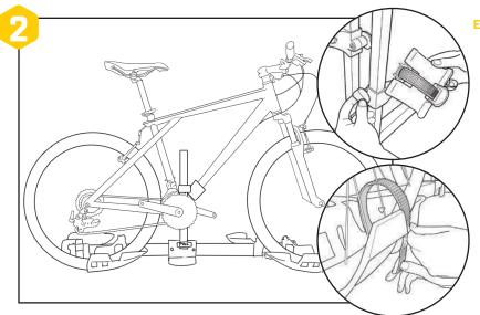
**EN** Secure bike wheel straps and down tube cradle.
