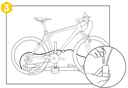
**EN** To lock bikes, use provided locking cable to lock bikes to vehicle's hitch.
