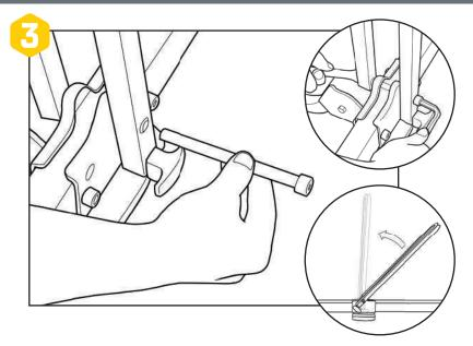
EN Secure upright with M10 x 120 bolt and nut using 17mm (9/16") wrench and 8 mm hex key.
