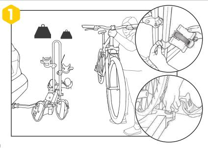
**EN** Load bikes. Heaviest bike closest to car. Adjust wheel tray if necessary. Tighten wheel tray knob.
