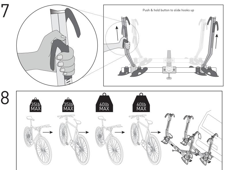
Load bikes, adjust wheeltray A if necessary, tighten knob.
