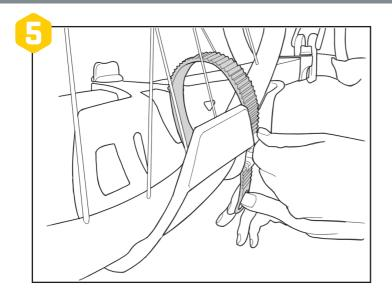
Use straps to secure front and rear wheels to trays.
