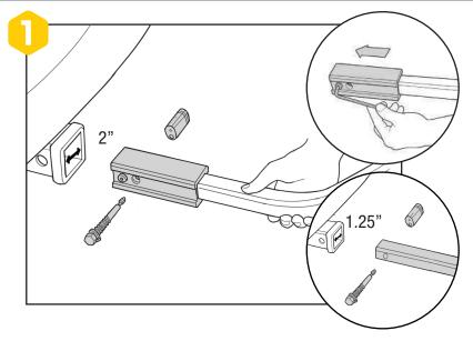
EN Install receiver and secure with pin and lock.
