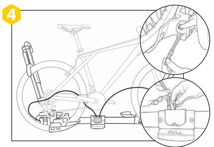
EN To lock bikes press and hold button, pull out lock shank. Be sure lock is in unlock position before inserting lock shank. To return cable press and hold button.
