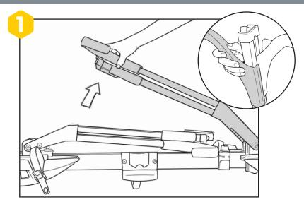
EN Push and hold button to open arm. Push and hold button to slide hooks up.
