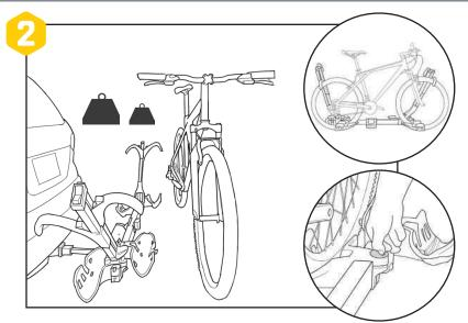
EN Load bikes. Heaviest bike closest to car. Adjust wheel tray if necessary. Tighten wheeltray knob. NOTE: Position arms at "10:00" and "2:00" without contacting bike frame
