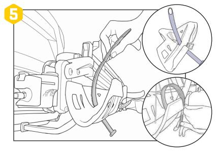
**EN** Thread Wheel Strap from bottom through strap slot. Click strap into place. Use Strap to secure rear wheel to tray.
