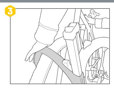
EN Press hooks down onto tires. Once the hook contacts the tire, fi rmly press the hook down until you hear 1 additional click. Ensure the tires are properly infl ated and in good condition.
