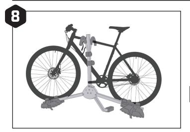
Adjust trays to fit the placement of bike(s) so that the bike(s) sits completely within the trays. Tighten knobs.
