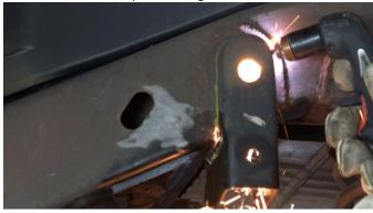
Begin cutting away the track bar bracket as close to the frame rails as possible.
