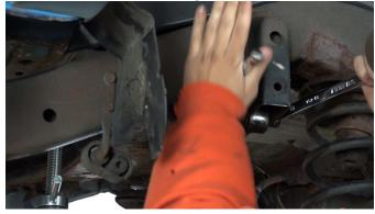
Remove track bar from the bracket. Down and out of the way.
