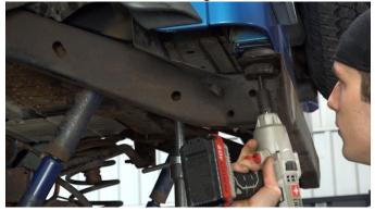
Depending on how you intend to cut, clean the cut zones free of rust and down to bare metal.
