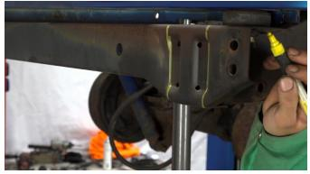
Depending on your level of experience, you may want to cut just outside of the frame rail to avoid cutting the frame. This will require you to remove any excess metal, such as welds, from the frame rails.
