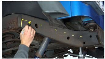
Measure 1.5" from the top of the vehicle's frame and draw a line. You will do this on the inside and outside of the frame rail.
