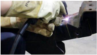
Begin cutting away the upper control arm mount bracket as close to the frame rails as possible.
