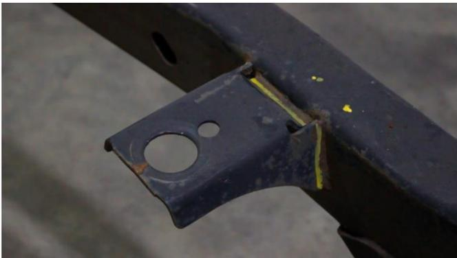
Begin cutting away the body mount brackets as close to the frame rails as possible.
