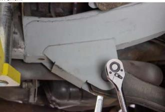
Reinstall upper control arm using 17mm socket.
