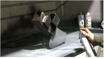
(OPTIONAL): Coat the part with a weld-able primer or other rust inhibitor to help prevent or reduce the risk of rust formation.
