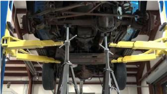
Remove lower control arm bolt from frame side bracket using a 21mm socket and 21mm wrench.
