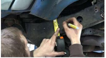
Using a tape measure, measure in from the front body mount bracket 1.5 inches and make a mark using a paint marker.
