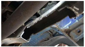
The part may fit snugly and require force. Ensure the frame rail is flush and the lower control arm bolt holes measure 57'' + -.5'' from center of front bolt hole to center of rear bolt hole.
