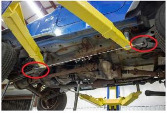
NOTE: If you have trouble getting the upper control arm bracket around the front exhaust section separate the front and rear exhaust sections to allow the front to flex.
