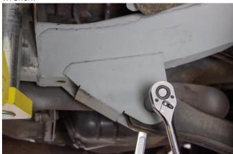
Reinstall upper control arm using 17mm socket.
