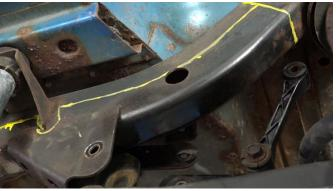
Depending on how you intend to cut, clean the cut zones free of rust and down to bare metal.
