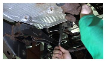
Mark down 1.5 inches from the top of the frame rail, on the inside and outside. You will need to cut off the frame side upper control arm mount on the inside of the frame rail.
