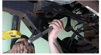
Remove upper control arm bolt using 15mm socket.
