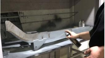
(OPTIONAL): Coat the part with a weld-able primer or other rust inhibitor to help prevent or reduce the risk of rust formation.
