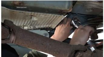
Reinstall the six transfer case skid plate bolts.
