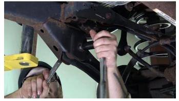
Remove upper control arm bolt using 15mm socket.
