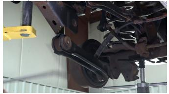
Remove upper sway bar end link bolt using an 18mm socket.
