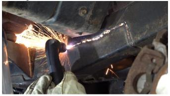
You will need to cut a small gap at the back of the body mount bracket and engine mount bracket to slide your new leaf spring mount section behind the brackets for welding.
