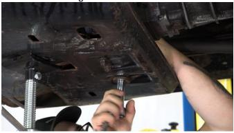
Support your skid plate with a jack or jack stand. Remove the six transfer case skid plate bolts using a 19mm socket.
