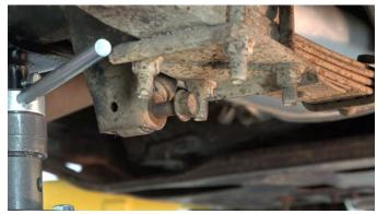
Remove the upper strut bolt connecting the shock to the Upper Rear Shock Mount and remove the shock.
