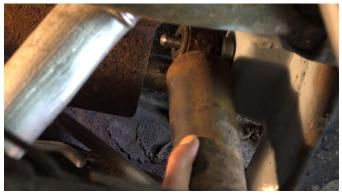
Reassemble the lower strut bolt and shock.
