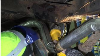
We recommend cutting the centermost support free first to allow easy access to the left and right support flanges, as well as the body mount bushings.
