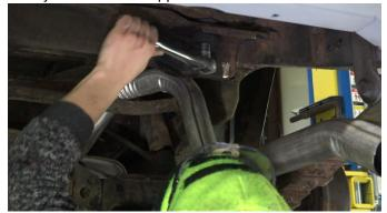
Depending on the exhaust routing, it may need to be removed or loosened to allow freedom of access to the tank support.
