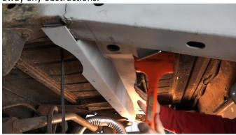
The part may fit snugly and require force. Ensure the frame rails are flush and the body mount bushing holes are aligned with the body.
