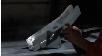
Replace the part and the body mount bushing. Reassemble the leaf spring with the included bolt, and resecure the body mount bolt. This will ensure the proper location of, and tension is applied to, the new part.
