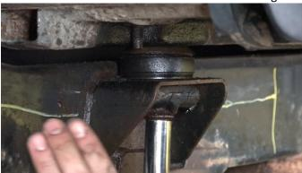
Remove the old bushing material and casing from the leaf spring. We recommend using an air hammer or hammer and chisel as it may be rusted and fused, making it difficult to remove.
