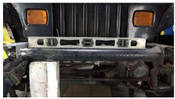
Replace the part to your measurements and Cclamp and tack weld it into place to prevent it from moving later.
