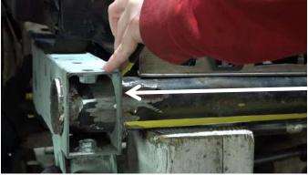
Take note of any difficulties and cut away any obstructions. The part may fit snugly and require force. If you have to bend the front cross member to fit the part into place, you may need to remove very small increments of material from the frame rail until it is flush. NOTE: Removing too much
