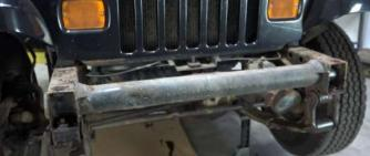
Using a T55 Torx, remove the front bumper, frame cover, and with a 10mm socket remove the cover support bracket.
