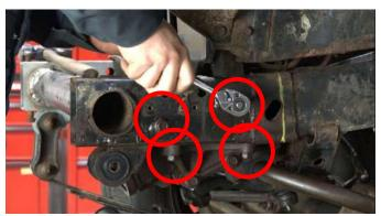
Using a 1-5/16" inch socket, remove the steering arm retaining bolt.
