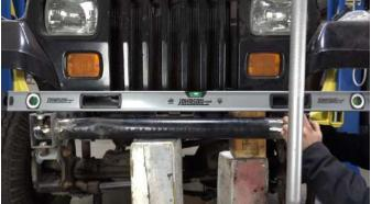
Replace the part to your measurements and Cclamp and tack weld it into place to prevent it from moving later.
