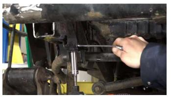
From the front edge of the OEM mount, measure 12.5" inches and draw a guide line around the frame rail. This line will be your cut line which avoids damage to the track bar bracket. If you intend on replacing this bracket, extra steps not listed will be required.
