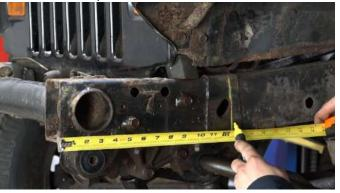
NOTE: The following steps require accurate measurements in order to allow correct amounts of weld-able frame.
