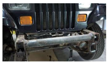
Using a T55 Torx, remove the front bumper, frame cover, and with a 10mm socket remove the cover support bracket.
