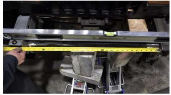
Take note of any difficulties and cut away any obstructions. The part may fit snugly and require force. If you have to bend the front cross member to fit the part into place, you may need to remove very small increments of material from the frame rail until it is flush. NOTE: Removing too much metal will make the gap size too large to fill with weld! Our part provides more material than what is needed for the install, per these instructions.
