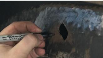
Continue to draw the line around to the inside of the frame, following the gas tank support, 1.5" from it and the top edge.
