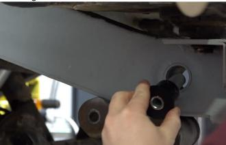
Using two 19mm sockets, rotate the shackle into place, send the bolt through, and secure the nut onto it. Reinstall your gas tank, cords, and tubes.
