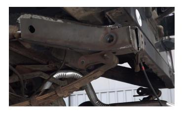
The part may fit snugly and require force. Ensure the bushing hole is visually aligned with the right side of the frame.
