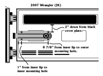
3. Mark the (4) mounting holes using the base plate as a template, and drill out with a small pilot drill bit, then enlarge using a ½" drill bit.
