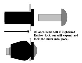
5. Tighten rubber lock bolts evenly to secure the Tailgate Stop to rear gate.
