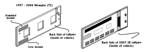
2. Locate the assembly on the rear gate using the diagrams provided for your year application. All measurement points are from the inner edges of the tailgate. It is important to make sure placement is correct or there could be interference with support ribbing inside of the tailgate.
