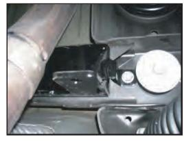
3. 2010-2011 vehicles will need to use supplied M10 bolt, Washer and Nut Plate to install mounting bracket. Slide nut plate on top of frame cross member. Place M10 spacer between frame and mounting bracket. Insert M10 bolr and washer. Start bolt into nut plate but do not tighten.
