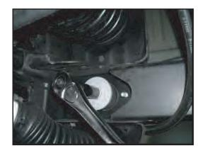
2. Slide the Mounting Brackets in between the frame and the exhaust. The muffler hangers may have to be removed to provide additional room. Position the mounting tabs of the Mounting Bracket onto the inner study of the body mount. Replace nuts removed in Step 1, but do not tighten.
