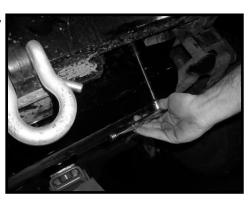
10. Move filler assembly into its correct mounting position and insert the 6 torx head screws to secure the assembly to the vehicle. Install license plate back into position. On the passenger side of the vehicle, reinstall the bracket removed in step 3 to hold the exhaust pipe in place.
