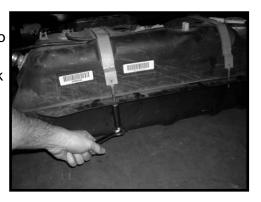
8. Position floor jack under vehicle with gas tank assembly centered on top. Slowly raise into position being sure to guide filler assembly to its appropriate location. Stop about 3 inches away from the skid plates mounting position and reconnect fuel and vapor lines. Also reconnect the electrical connector before lifting into final position.
