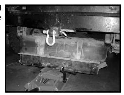
7. Locate the square cutouts in the RR skid plate and install the metal straps removed in step 6. Before fastening the straps, place the gas tank into the RR skid plate. Locate the proper slots in the RR skid plate for each straps threaded stud. Tighten the nuts onto the studs to secure the gas tank to the RR skid plate. Be careful not to over tighten these bolts.
