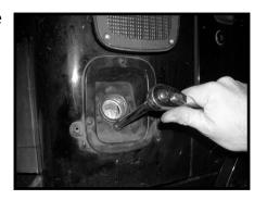
3. Remove the nut from the bracket holding the exhaust pipe in place on the passenger side of the vehicle. This will allow movement in the exhaust pipe during removal of the tank from the vehicle.
