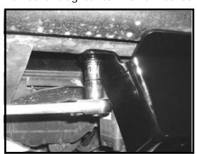
9. Tighten the lower bumper and lower frame to 65 ft-lbs and the cross member bolt to 20 ft-lbs.
