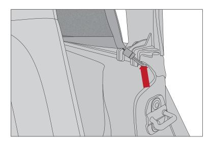
4. Hook two bottom bungees to openings in tub rail as shown on right. Repeat for second side.
