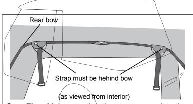
**Step Five:** Make sure that the straps sewn into the rear of the top are behind the rear bow.
