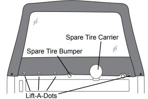
**Step Nine:** Fasten the bottom of the Rear Curtain to the Lift-A-Dots on the rear of the vehicle.
