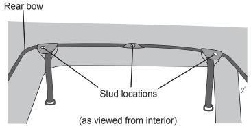
**Step Three (Optional):** If the Studs are missing from the top bow, install Body Studs (not included). Center the rear seam on the bow and use the snap flap as a guide for marking the location of each snap. Center punch and drill a 3/32" hole for each stud. Install the studs with a sheet metal screw.
