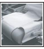
10. Test all seat functions. Hooks and straps should not effect seat movement.
