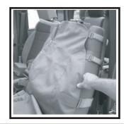
7. Attach top hook and loop fastener strap and front hold down strap to back cover.
