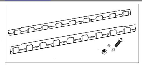
NOTE: These rocker guards have been designed to fit the contours of the vehicle. Instructions must be followed to insure the correct placement and adhesion of this part. If surface is not cleaned and prepared as stated below proper fitment will not take place. Do not install if outside temperature is below 65F or above 100F. Allow part to sit overnight before driving.
