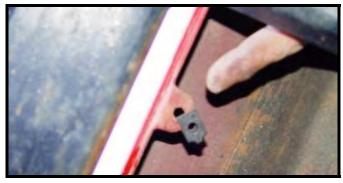
**Step 5:** Position armor onto lower side rocker panels. Make sure that it is evenly spaced before applying any pressure to armor. When satisfied with placement apply pressure to all areas to properly secure armor to vehicle. Secure bottom of rocker guards with hardware supplied.
