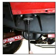
**Step 5.** Once all the nuts have been tightened, tighten the center bolt of the body mount to 80-ft/lbs. Repeat for each mounting location.
