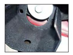
**Step 4.** Once all the nuts have been loosely threaded and the Guard is attached to the vehicle, begin tightening the nuts to 40-ft/lbs. Repeat for each mounting location.
