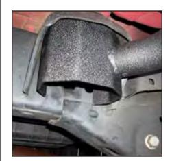
Step 3. Supporting the RRC Side Armor from underneath, lift the Armor into place and slide it between the large washer and the body mount, taking care to align the holes in the Armor mount with the two body mount studs. Apply several drops of threadlocker to the studs. Thread the two nuts onto the studs loosely. Repeat for each body mount location.
