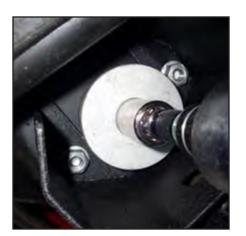
**Step 2.** Once the center bolts are removed, remove the remaining two (2) 16mm nuts located on either side of the bolt. Do this for each of the four (4) body mounts.
