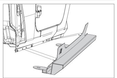
**NOTICE** Have someone help lift the Rock Rail into place to avoid damaging the vehicle.
