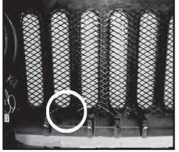
Step 3. With the grille insert matched to the opening of the grille use one of the braces to mark the mounting holes to be drilled. Hold the brace between the 1st and 2nd grille cutout on the left side.
