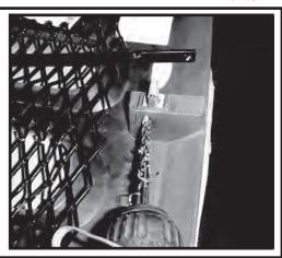
Step 5. With the lower portion of the brace secure apply pressure to the brace and mark the upper mounting holes. Using a 3/16" drill make a hole. Use low RPM when drilling the holes. Hole should be a minimum of one inch from the top edge of the grille. Using a supplied bolt and nut secure the brace to the grille. Do not tighten at this time. Repeat for other brace.
