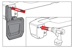
6. Attach splash guard with short phillips head screws.
