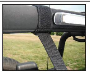
Step 1. Place LED light against the roll bar and wrap both straps around the bar and feed them through the plastic buckles.
