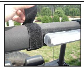
Step 2. Pull the slack out of the straps and wrap around to attach the strap.
