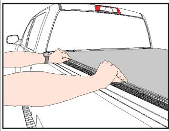
Engaging Hook and Loop, <u>Step One:</u> After rolling the cover closed, grab the fabric loop flap and evenly pull loop over the hook track engaging the loop to the hook track. Avoid pulling fabric flap straight up.
