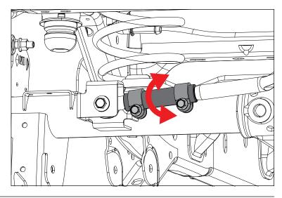
6. Once centered, tighten adjustment bolts and torque to 45 ft.-lbs.
