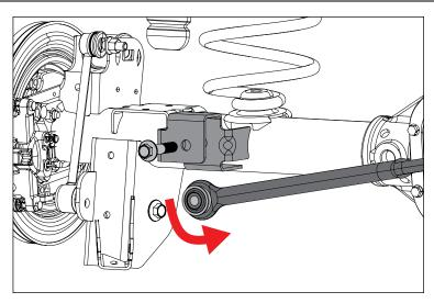
2. Remove rear track bar from frame bracket.
