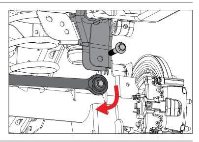
3. Loosely install Adjustable Rear Track Bar in frame bracket using factory hardware.
