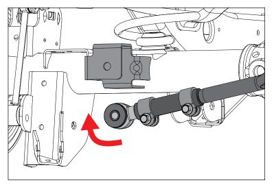
5. Center axle by loosening adjustment bolts and turning adjustment sleeve.
