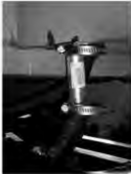
Insert fuel extension pipe in the hose. Tighten hose and extension down with hose clamps from the body lift kit.
