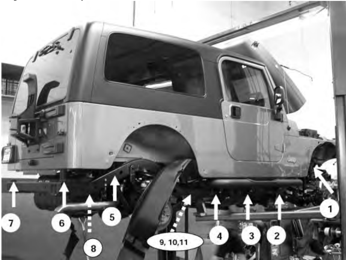
Picture shows position of the of the body pucks. Body pucks 9 – 10 – and 11 are the opposite side of 4-3-and 2.
